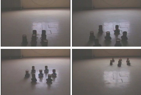
Fig. 1 Seven robots form a hexagon, and move towards a light source.
