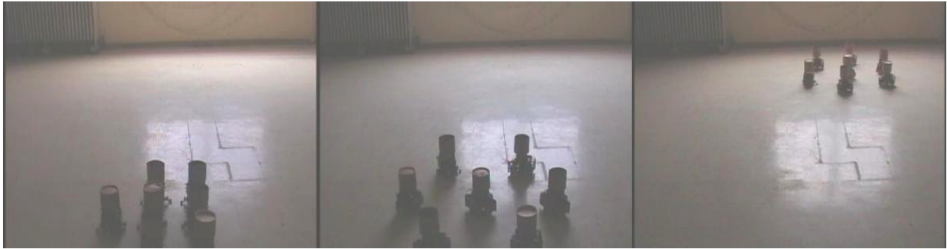
Figure 1. Seven robots self-organize and move in formation to a light source. Each robot is autonomous.
