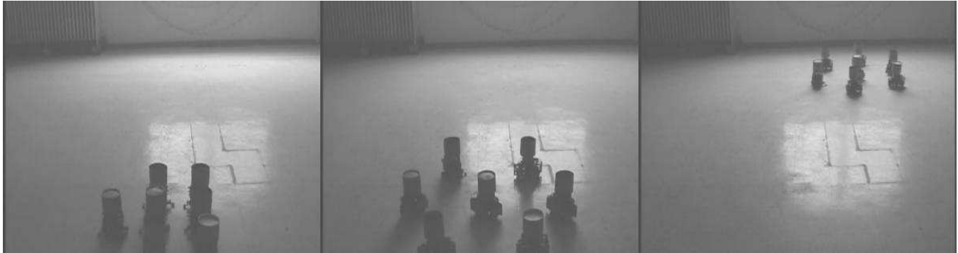
Figure 1. Seven AP robots self-organize and move in a hexagonal formation toward a light source. Each robot is autonomous.
